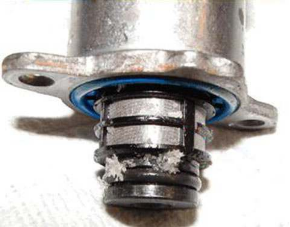
LGH/LML Fuel Pressure Regulator 1 Contaminated With DEF
