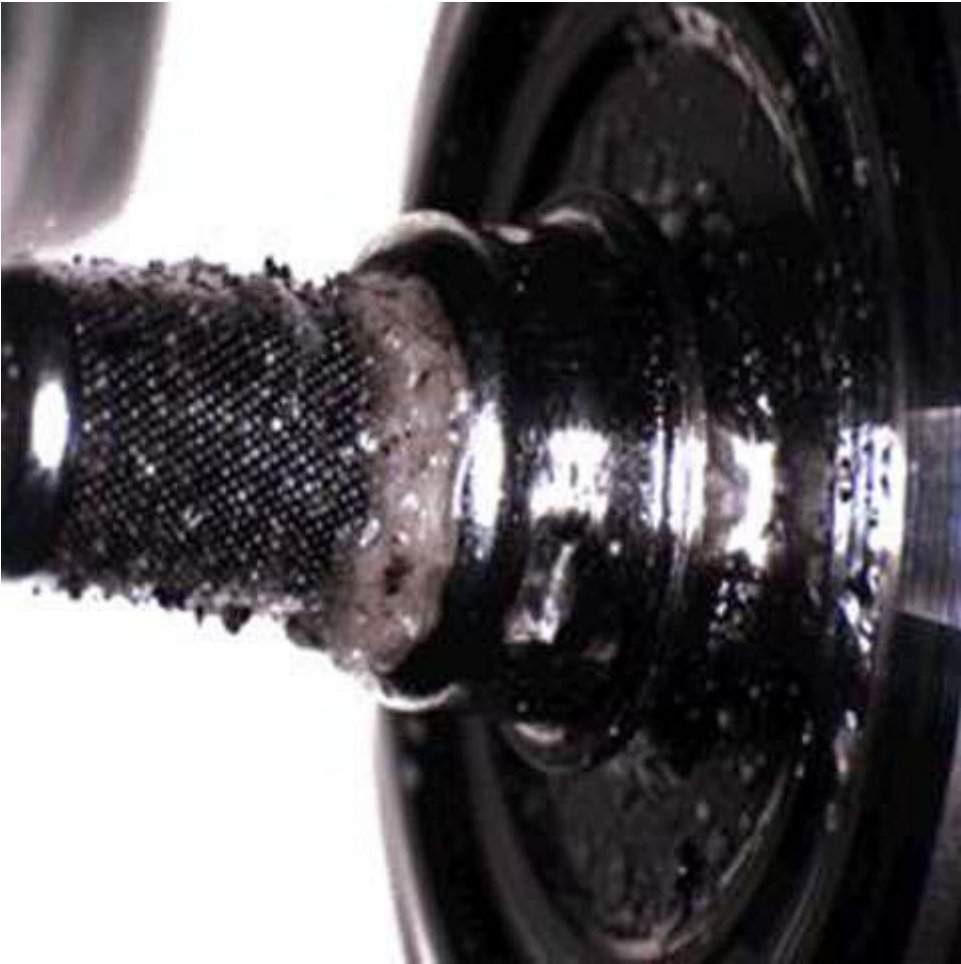
LGH/LML Fuel Pressure Regulator 2 With DEF Contamination
