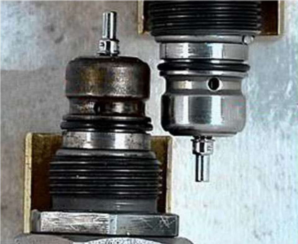
LGH/LML Fuel Pressure Regulator 2 With Rust (On Left) Due To Water Contamination
