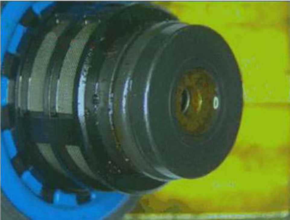
LGH/LML Fuel Pressure Regulator 1 With Rust Due To Water Contamination
