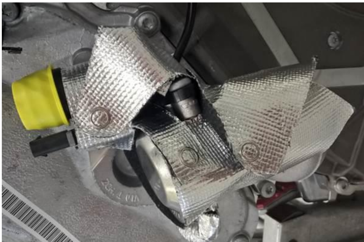
Figure 2. Insulation on Bank 2 pressure sensor after installation.
