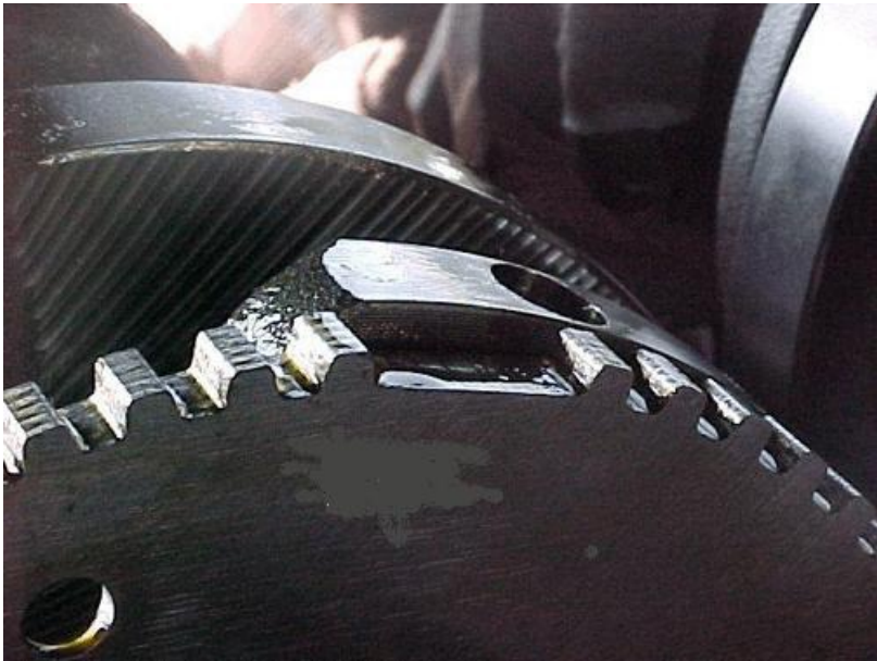
Crankshaft with bad reluctor wheel.
