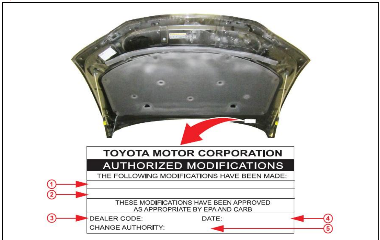
Figure 1. Location of Authorized Modification Label for 2015 RX 350
