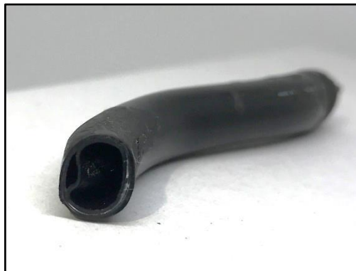
Restricted Fuel Line
