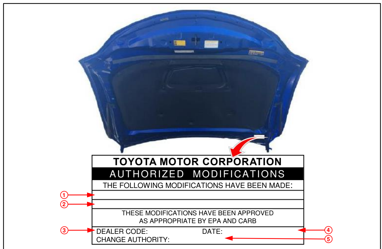
Figure 1. Location of Authorized Modifications Label on 2016 – 2019 RX350 and RX350L
