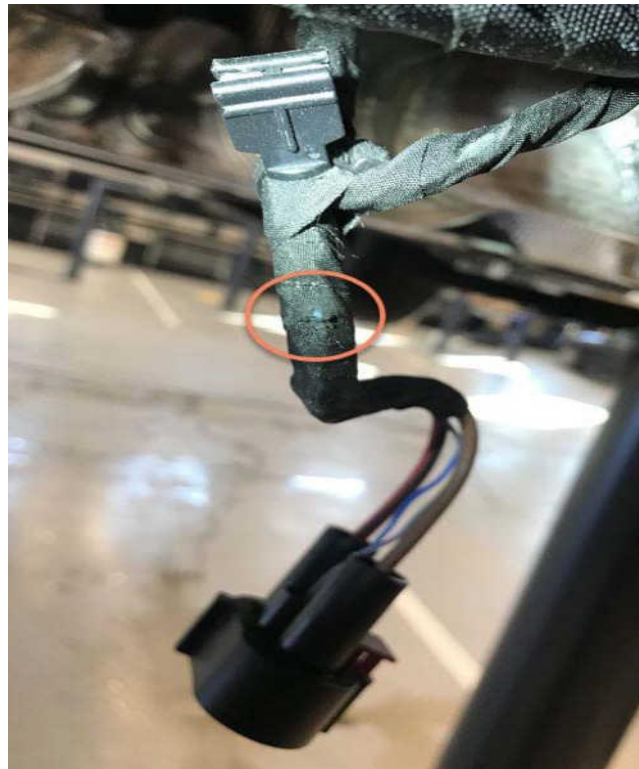
Figure 3. The damage on the original harness might be difficult to spot.
