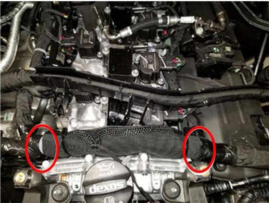
Example of engine wiring harness damage at Camshaft Carrier Cover shown below.
