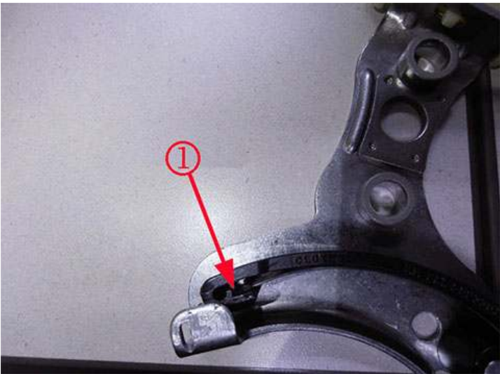
1) Short spring not reaching the pivot
