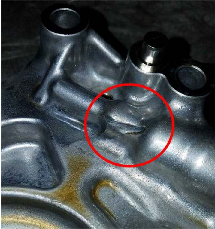
The hole in the oil pump
