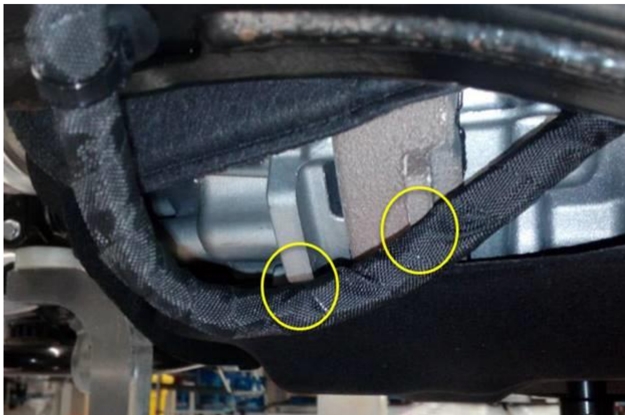
Figure 3. Inspect for potential chaffing between the transmission lugs and the harness.
