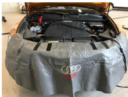
Figure 2. Protective workshop cover.
