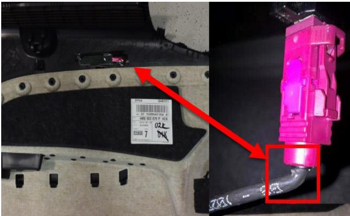
Figure 2. Coaxial wire kinked at R263 SOS Antenna.
