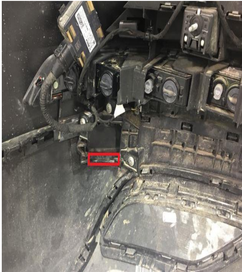
Figure 3. Bracket part number located on passenger's side.
