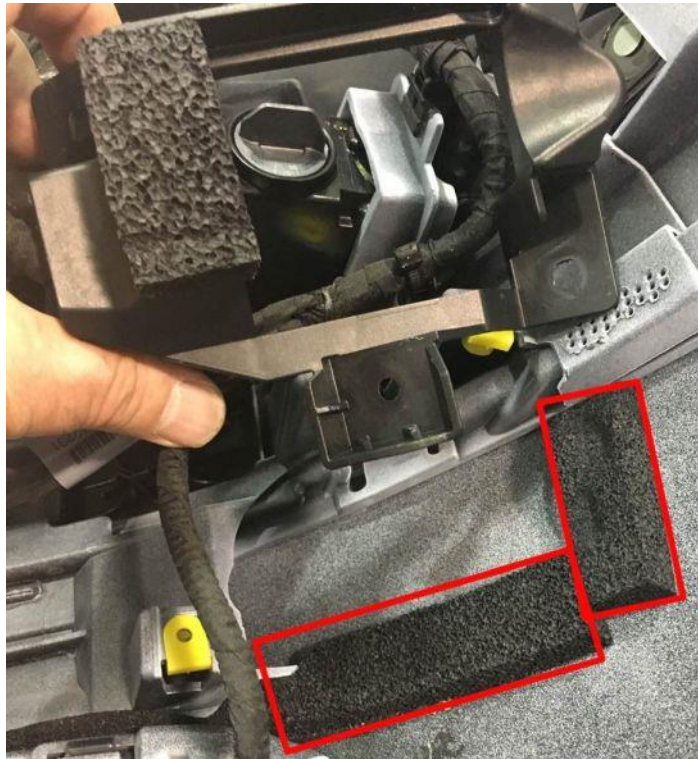
Figure 4. Foam to be stripped out.
