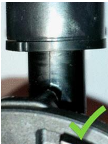
Figure 6. Correctly-installed sensor and grommet.
