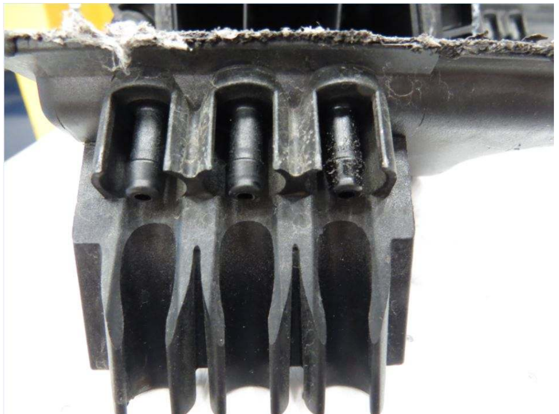
New vacuum reservoir output ports.JPG:
