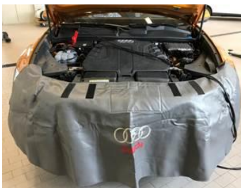
Figure 2. Protective workshop cover.
