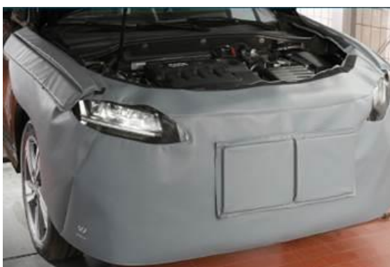
Figure 3. Protective workshop cover.
