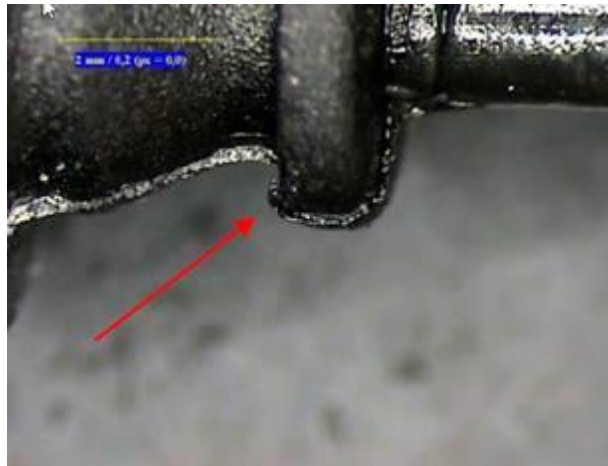
Figure 4. Burrs that need to be removed.
