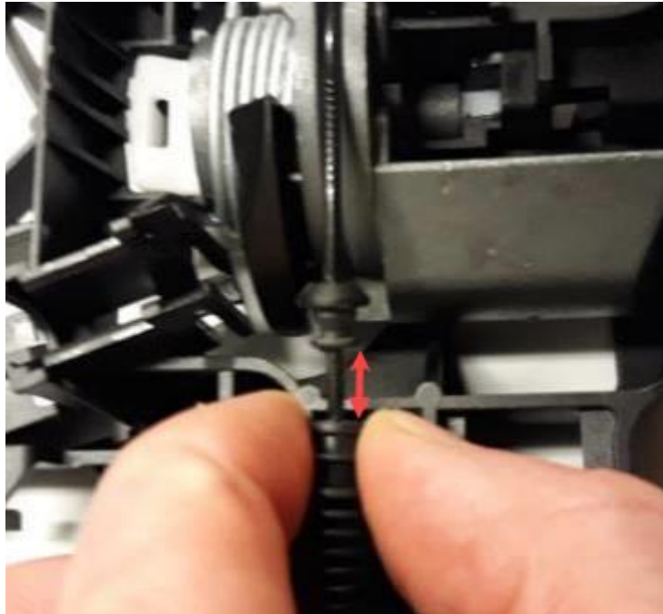
Figure 2. Separate the boot from the cable retainer.
