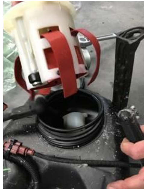
Figure 1. Filter element housing is loose inside the tank.
