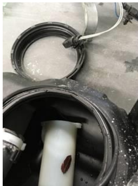
Figure 2. Filter element housing is loose inside the tank.
