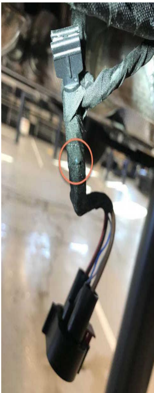
Figure 3. The damage on the harness might be difficult to spot.
