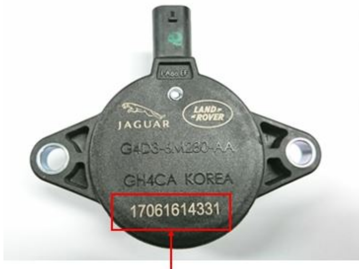
Part Serial Number – Breakdown from left to right
