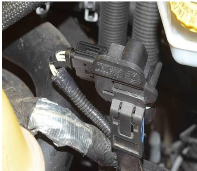
Fig. 4 New Differential Pressure Sensor Reinstalled
