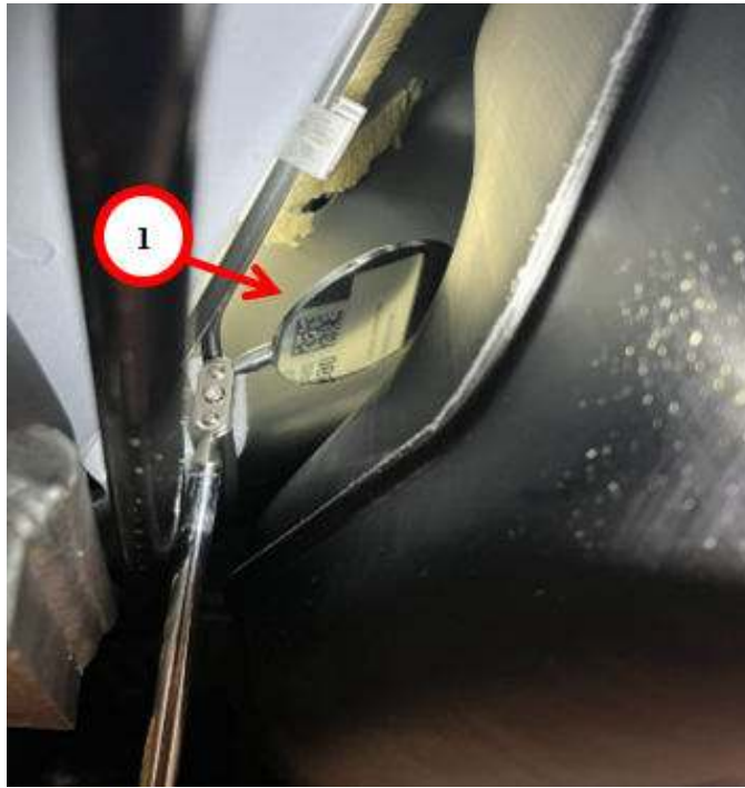
Fig. 3 Mirror Capturing Parts Label On Fuel Tank
