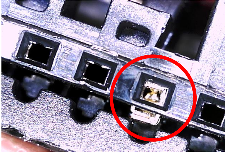
Misaligned Terminal In IP Harness D3944A
