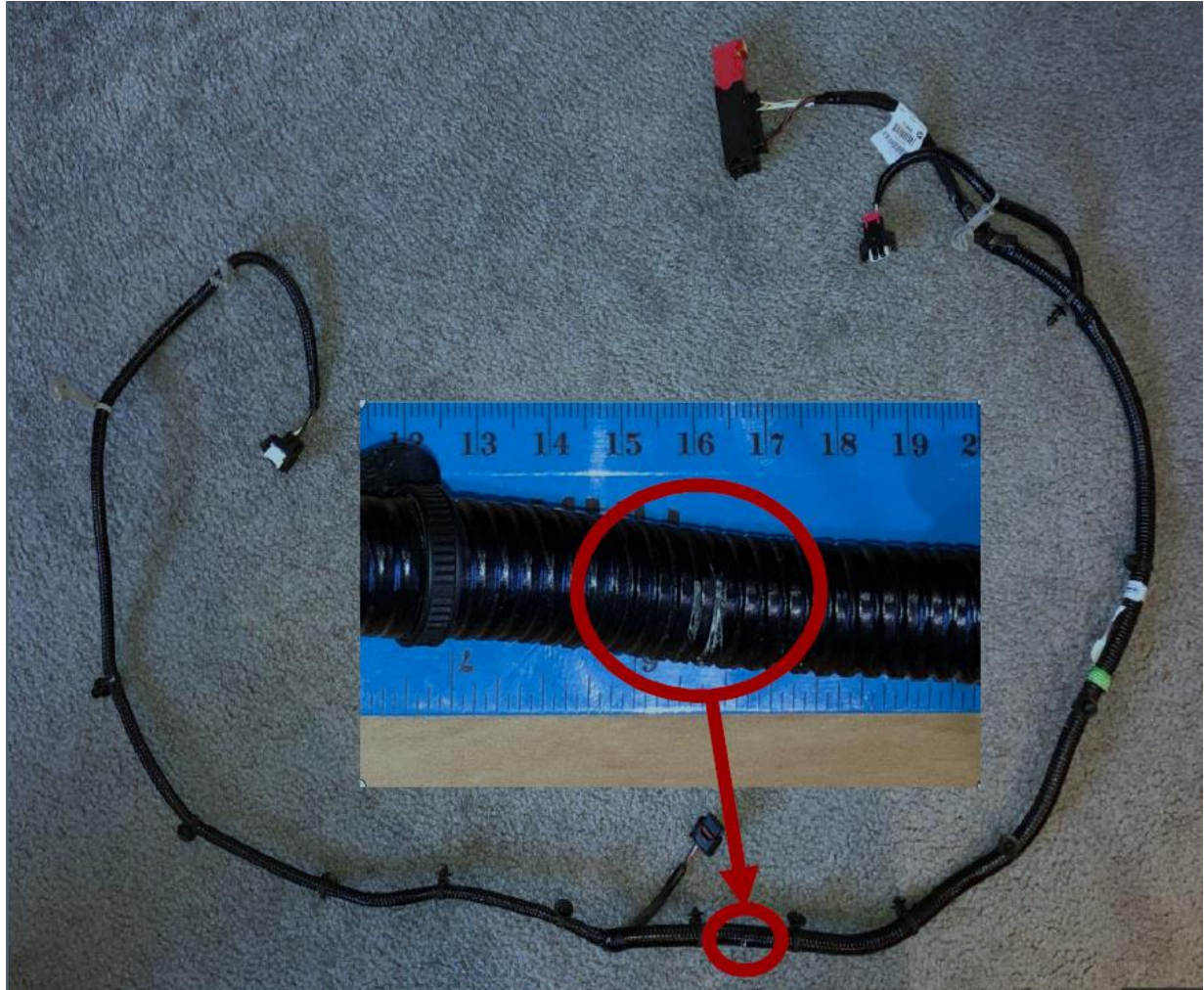
Damaged AGS Wiring Harness
