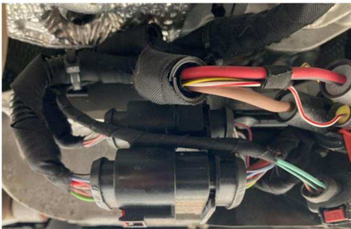
Figure 1. Connectors in the wrong position.
