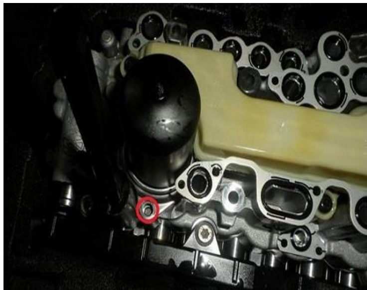
Figure 5. Bolt head is missing.
