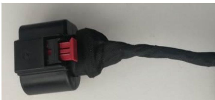
Figure 5. Completed harness wrapping.
