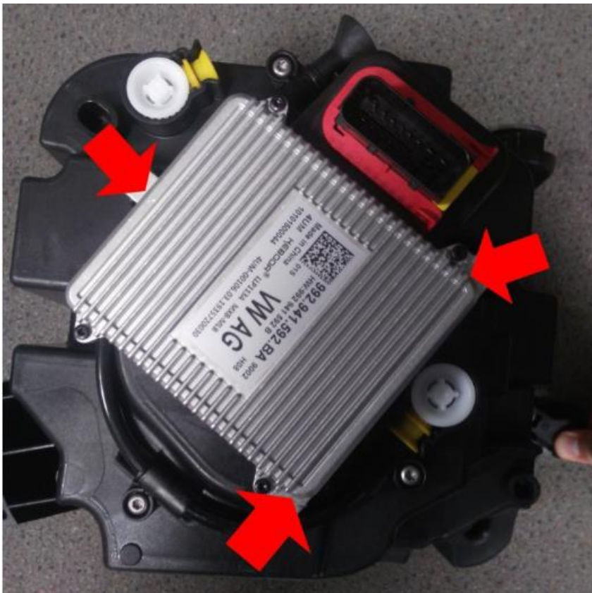
7) Referring to Figure 9 – Refit the three screws and secure to 2.0 Nm
