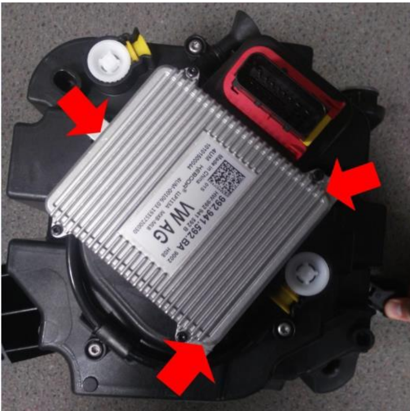
Figure 2 3) Referring to Figure 3 – Gently pull up the module and slightly pull the harness to make it free as shown in Figure 4
