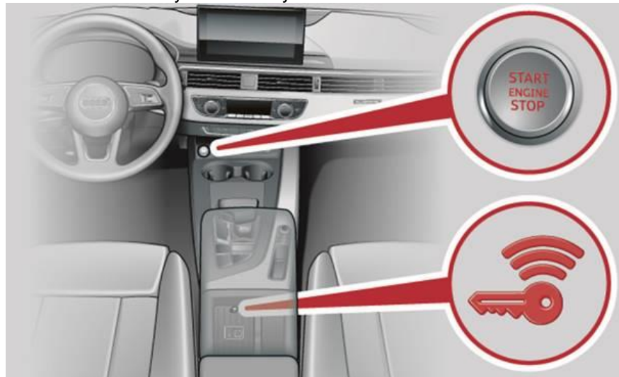
Figure 2. Location of the key reader coil.
