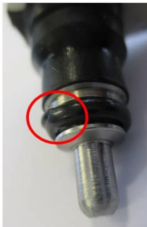
Figure 1. O-ring is pinched.
