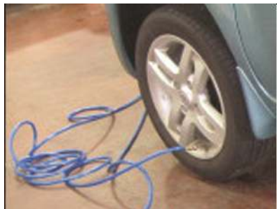
Long heavy hose with Lock-on air chuck or wheel at 6 O'clock position
