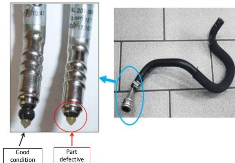
Figure 1. Good condition part or defective part.
