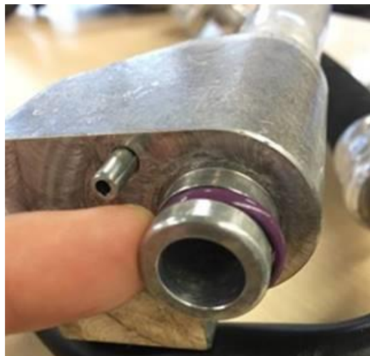
Figure 1. Damaged refrigerant line O-ring seal.
