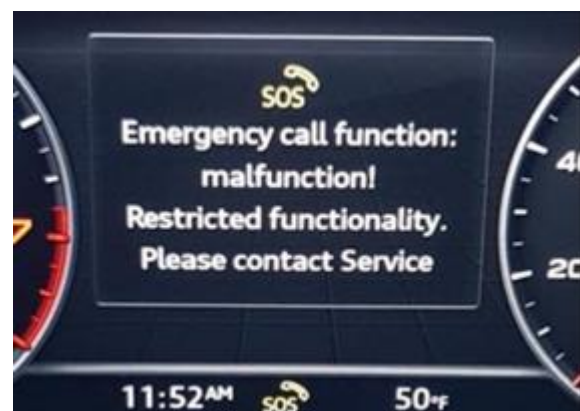
Figure 1. The warning message is shown in the instrument cluster.
