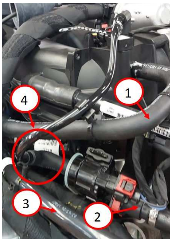
Fig. 1 Kinked Purge Line Elbow
