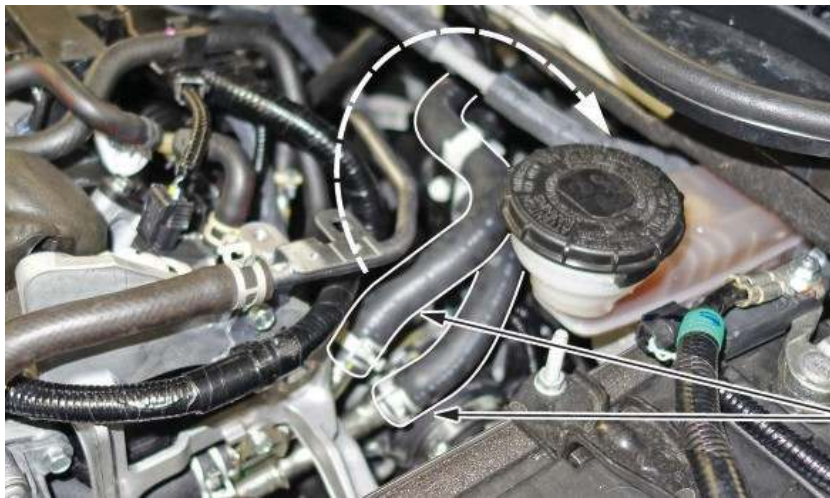
HEATER HOSES Disconnect and swing up and out of the way.
