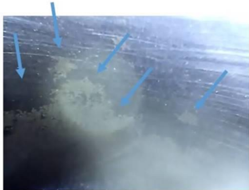
Figure 2. Corrosion marks on cylinder walls (close-up).
