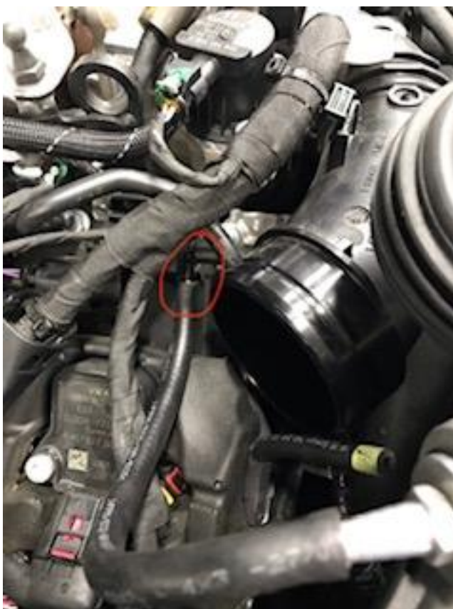
Figure 2. The output port of N649 (close-up picture).
