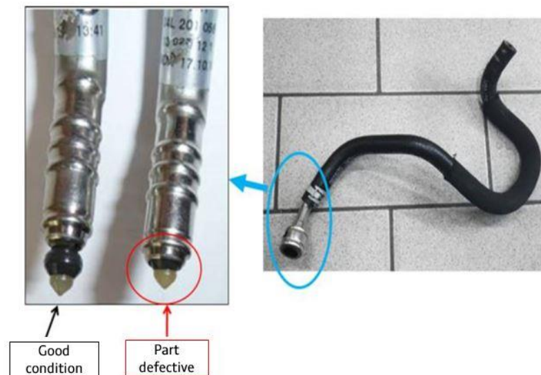
Figure 1. Good condition part or defective part.
