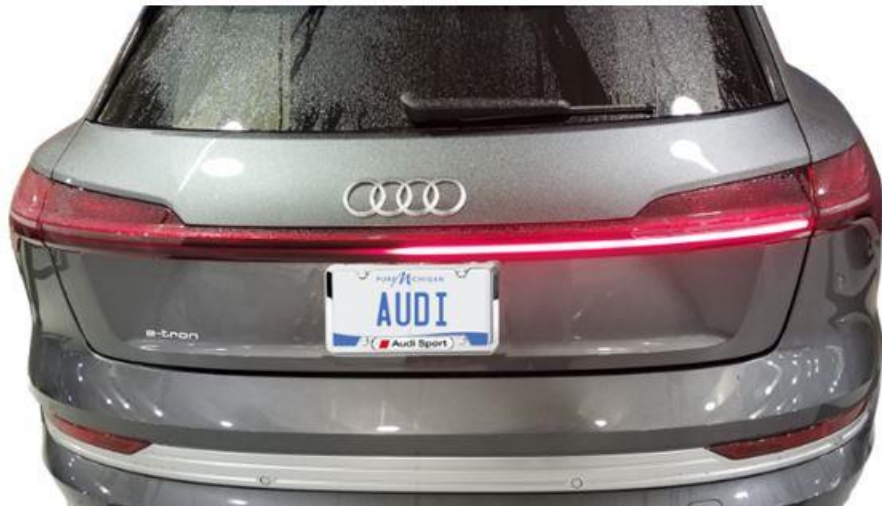
Figure 1. Partially lit trunk lid taillight.
