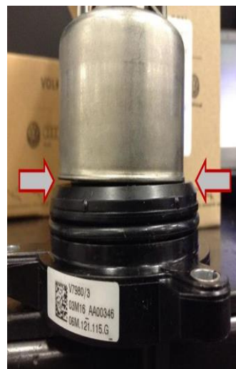
Figure 1. Gap between chamber and seal.
