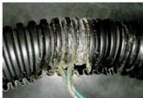
Corrosion residue/debris and damaged circuit insulation are visible at the takeout point of D1575A.
