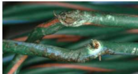
Magnified view of damaged and corroded wires near connector D1575A takeout point. Note that several strands are broken
