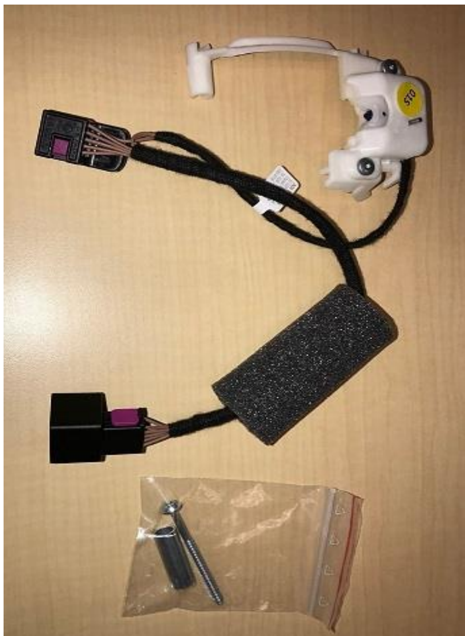
Figure 1. New microswitch module.
