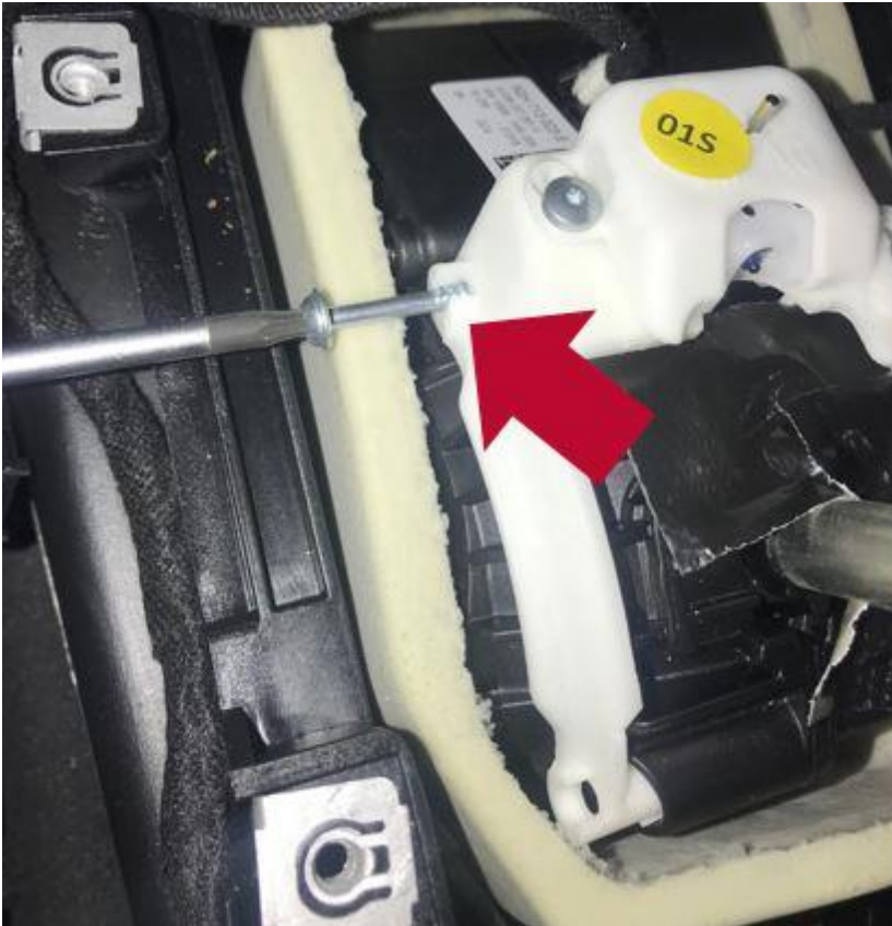
Figure 8. Installation of the screw.
