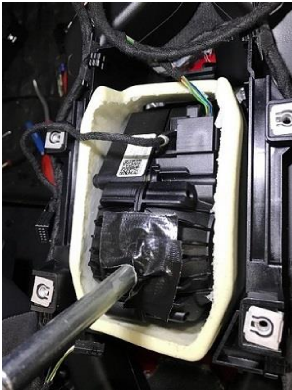
Figure 3. Tape covered shift gate.
