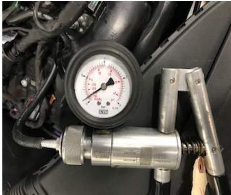
Figure 1. Checking the vacuum at the output port of N649.
