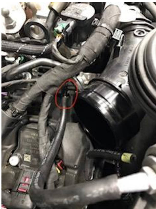
Figure 2. The output port of N649 (close-up picture).
