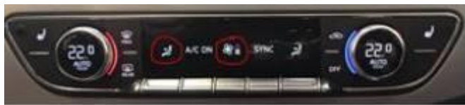
Figure 8. 72°F (22°C), Sync, air distribution to central vent, medium blower speed.
