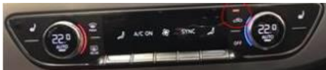
Figure 5. Auto, 72°F (22°C), Sync, air recirculation mode.
