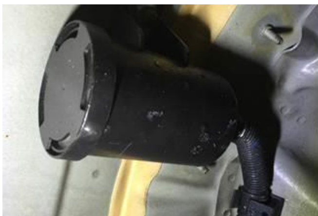
Figure 10. Remove original NVLD filter.
