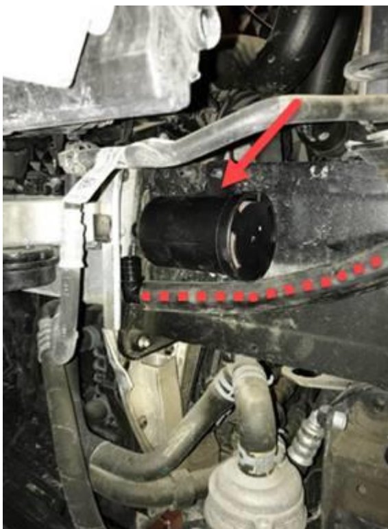
Figure 3. Installing the new NVLD filter.
