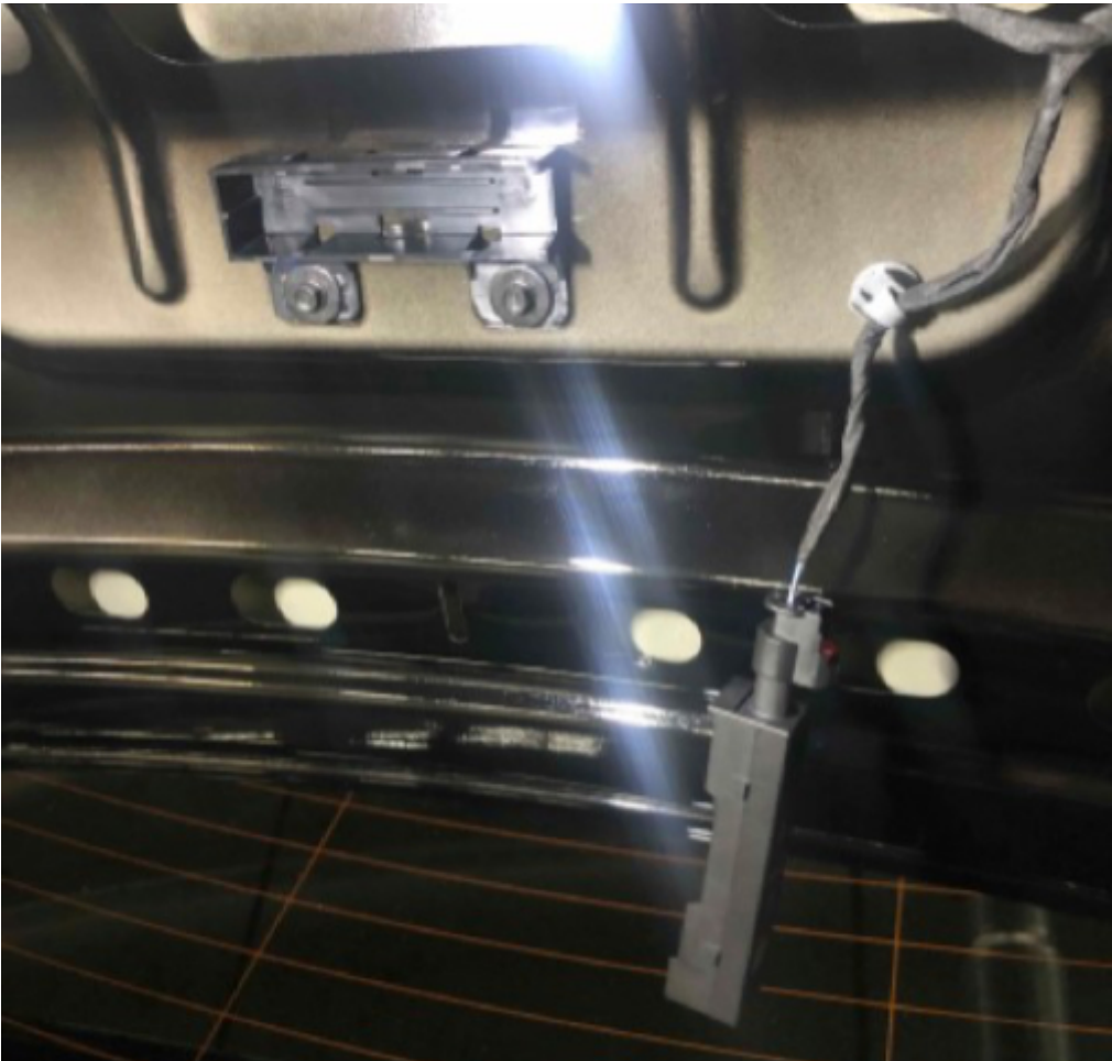
T10E Keyless Entry Antenna - Rear Compartment
