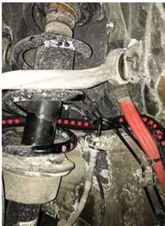
Figure 6. Routing the rubber hose.
