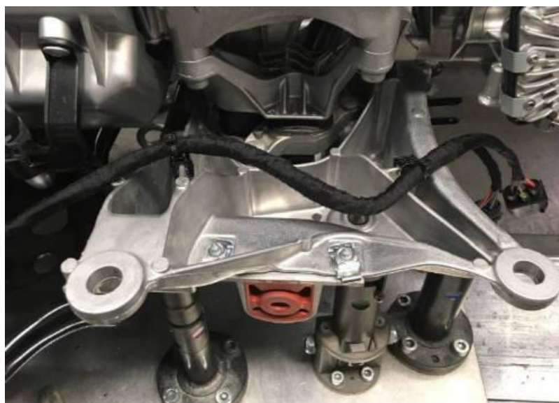
Figure 8. Routing and mounting of the transmission harness behind the crossmember.
